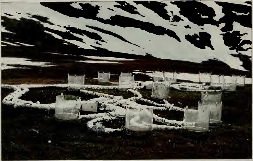
Fig. 7. CO 2 -enrichment experiments in the Swiss Alps at 2500 m elevation. Elevated CO 2 did not stimulate plant growth, but affected plant quality and biodiversity, though only slightly, suggesting a very slow response (Körner et al. 1997).
